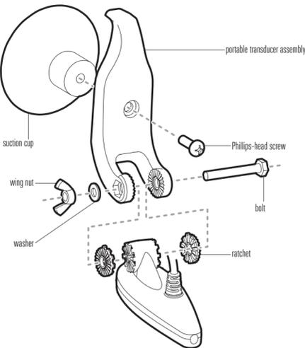
**NOTE:** If you are unable to ratchet the transducer so that it rests below the water, you can disassemble it and align the beads with a different number until you reach a position that allows the proper alignment.
