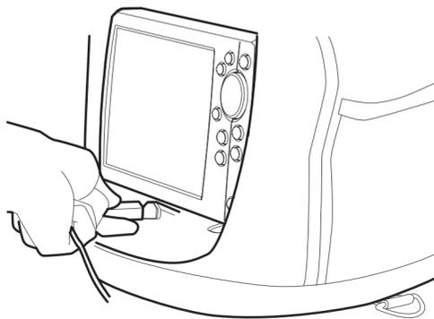
**Speed Accessory (Optional):** If you are installing the optional Speed Sensor accessory, insert the Sonar/Speed Y-Cable connector into the jumper port in the portable case. Then, connect the transducer connector and speed sensor connector to the corresponding connectors on the Y-Cable. The Y-Cable requires a separate purchase. Contact Humminbird Technical Support for details.
