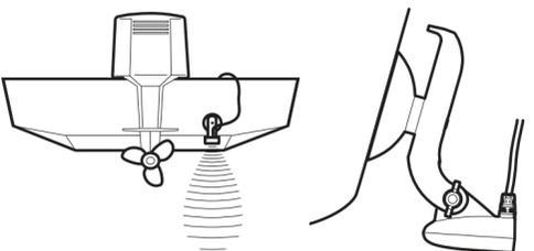
3. Hand tighten the wing nut so that the transducer will not rotate.
