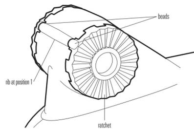
2. Assemble the other transducer parts as shown (see the illustrations **Assembling the Plastic Bracket**). Hand tighten only!
