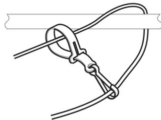
5. When you have finished using the transducer, unplug the transducer cable from the transducer jumper port on the base, then coil the cable around the assembly.
